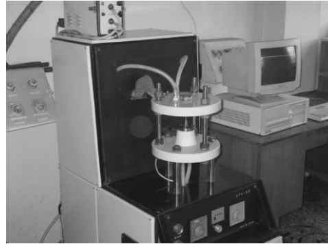
Fig. 2. Equipment for the study of low-cycle or multi-cycle fatigue
