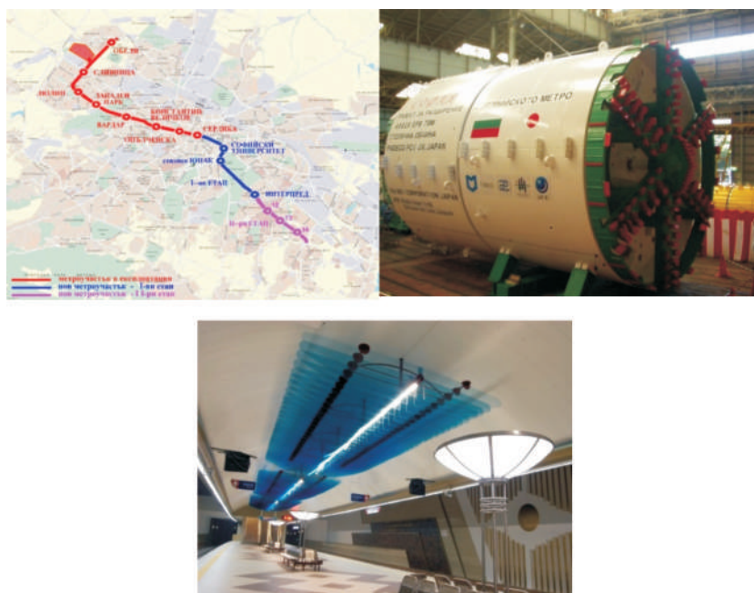
Fig. 4. Scheme of Line 1 in 2009. Tunnel Boring Machine 6 m of diameter for the construction of tunnels in section MS Serdica – MS V. Levski Stadium. View od MS SU St. Kl. Ohridski
