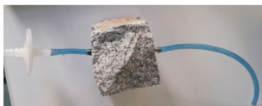
Fig. 2. Preparation of measuring hole ø6
