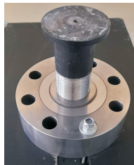
Fig. 8. Laumas Tensometer up to 100t
