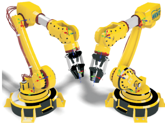
Fig. 1. A robotic arm with UCSs attached to each joint (render: Autodesk Inventor)
