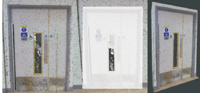
Fig. 1. RECAP Pro Example – Object is closed from point cloud, then clipped and clipped area reduced within the software using the Limit Box Function, and then solidified using the “Scan to Mesh” tool. This can then be brought into REVIT as an object
