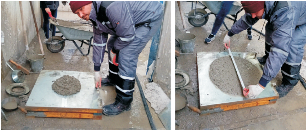
Fig. 2. Measuring the consistency of concrete mixture by means of the flow table method according to EN 12350-5
