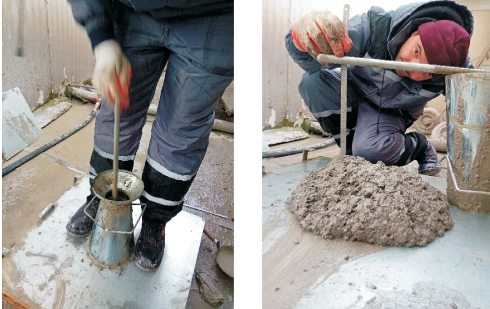
Fig. 1. Measuring the consistency of concrete mixtures by the slump method according to EN 12350-2
