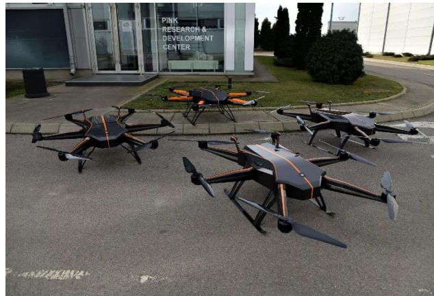
Fig. 1. Multicopters IKA-20 that can carry 20 kg of payload [3]
