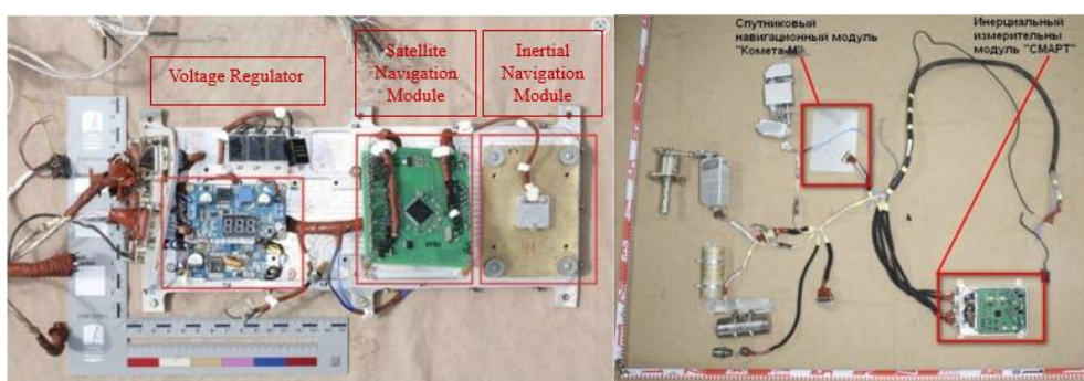
Fig. 4. UMPK guidance unit components. Source: Black Mountain Analysis
