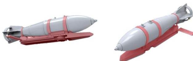
Fig. 2. UMPK Kit (highlighted) on the FAB-500 M62. Glide wings are folded. Source: Arma Models
