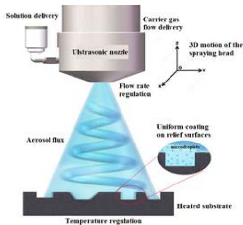
Fig. 3. Simplified representation of the spray deposition process, according to Siansonic spray coater machine design
